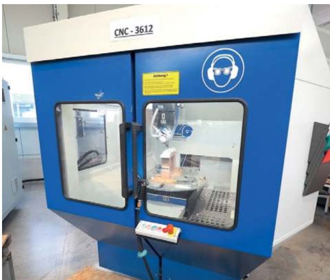
In use since 2018: The RT-F 1400 5-axis CNC rotary table milling machine for small workpieces
