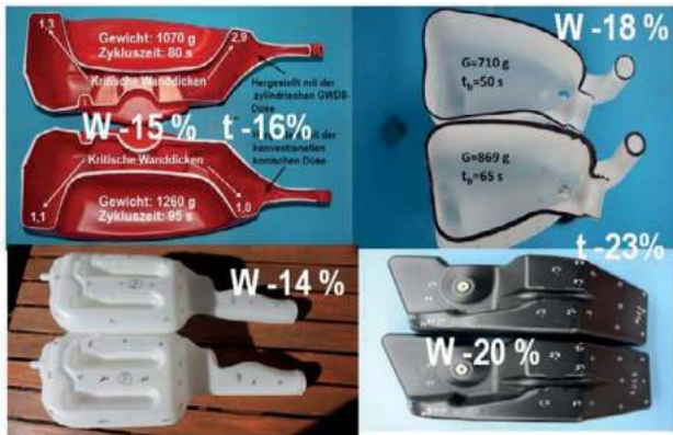
Picture 4: Articles that have been produced with a conventional conical die and with a predominantly cylindrical GWDS-die
