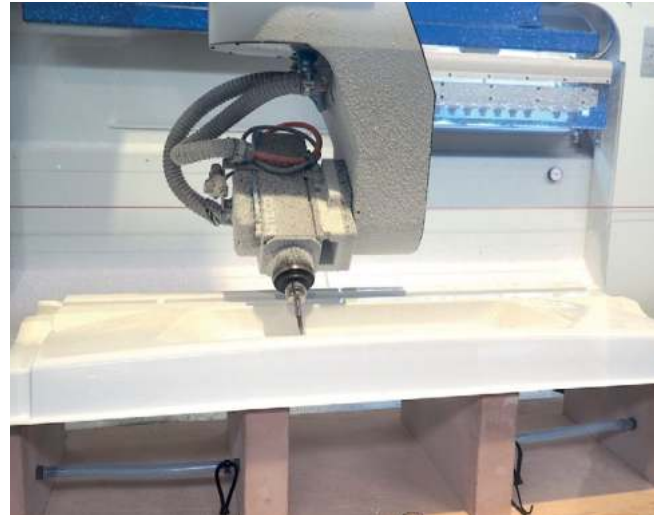
Around ninety percent of the technical parts that swissplast thermoforms in Gotha end up being milled
